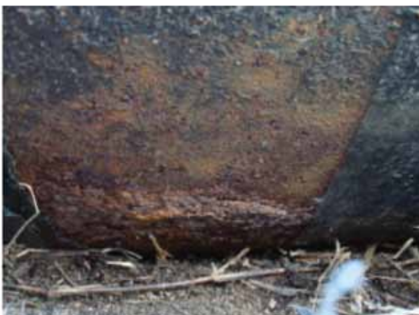
Figure 9: Corrosion patches revealed after removing the insulation at the location indicated by guided waves inspection.
