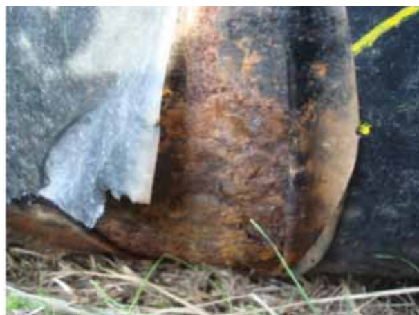
Figure 9: Corrosion patches revealed after removing the insulation at the location indicated by guided waves inspection.
