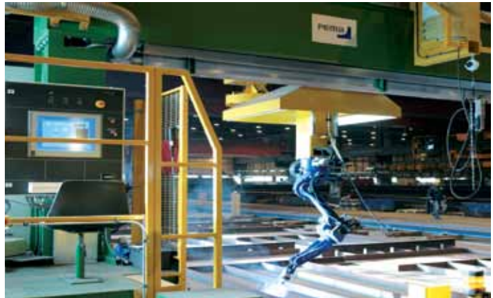
The VRWP-8000/1 Vision Robot System with a MOTOMAN-SSA2000 welding robot at the STX Turku shipyard – best suited to welding panels that are largely similar but not identical.
