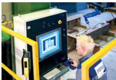
The robot operator can easily program the welding path based on the image of the scanned workpiece.
