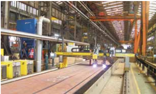
One of the high-tech Esab cutting systems bought by Genrec for use in the process of constructing boxed steel columns for power stations.
