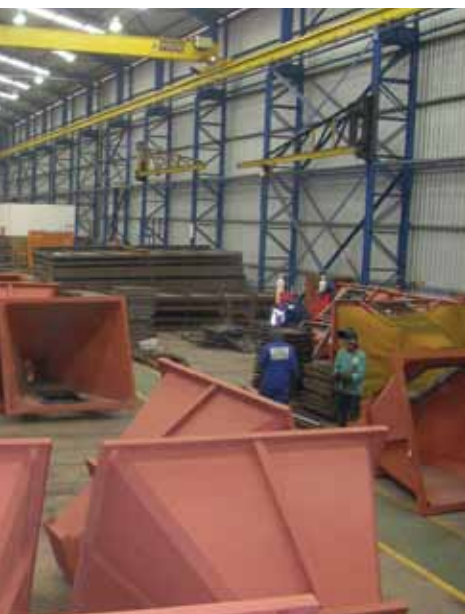
AGS Engineering's new Alrode facility – a 5 000 m 2 covered area with three 5-ton and one 25-ton overhead cranes – a facility for fabricating 350 tons of steel per month.
