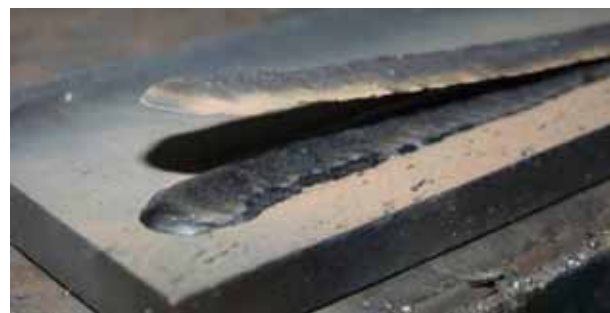
Figure 3: Self-releasing slag design of a flux cored wire – Böhler CM2 Ti-FD (E 91T1-B3M).
