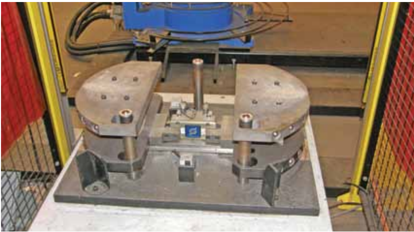
The ridge-locking mechanism is used to locate each muffler before being lifted by the handling robot.
