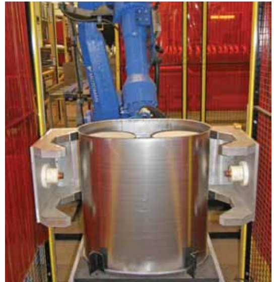
The gripper on the handling robot picks up the component to an accuracy of within 0,2 mm and the outside hold allows free access to all of the internal seams.
