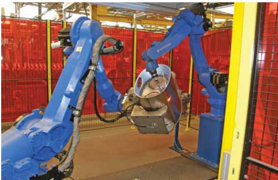
Jigless welding of CES mufflers using Motoman robots and SKS welding power sources. The handling robot and welding robot move simultaneously to access all of the internal seams. The process substantially improves reliability and cycle times, offers much better access to weld joints and cost savings over jig and manipulator-based systems.
