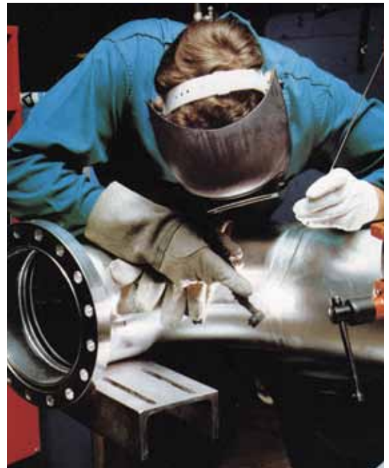
Aluminium welding requires more skill and attention to detail than does mild steel welding.
