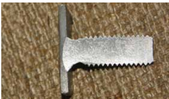
The drawn arc stud welding process results in welds on base metals that are stronger than the surrounding metal and have maximum weld penetration without marring the other side.
