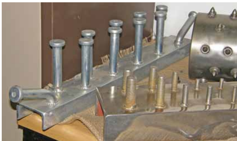
Stud welding test samples: "Studs are used in places that you would never know about," says Simpson.
