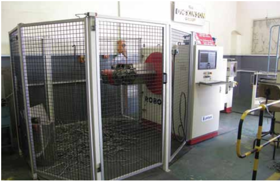
Refractory Fibre's CNC wire bending machine manufacturing stainless steel anchors for a rotary cement kiln.
