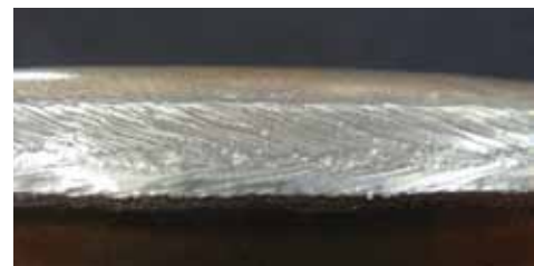
A weld on a pressure container performed using the Lincoln Power Wave i400 120 kHz inverter controlled by RapidArc software at 2,99 m/min (49,84 mm/s).
