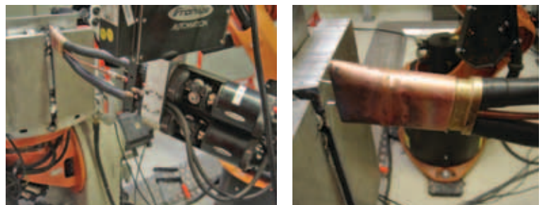
Figure 10: Regular twin-wire torch equipped with modified prototype gas nozzle [7].
