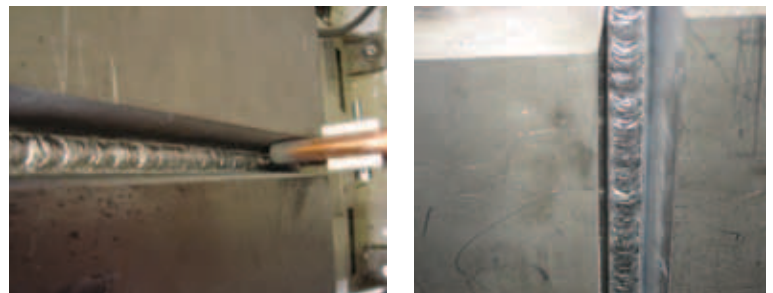
Figure 9: First 3G narrow gap root pass welded with twin-wire technology [7].
