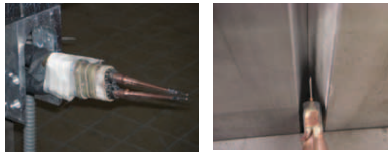
Figure 11: Modified twin-wire torch for narrow gap thick section aluminium high deposition welding in the 3G position [7].
