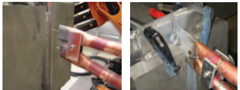
Figure 8: Initial trials using modified single wire GMAW welding torches [7].
