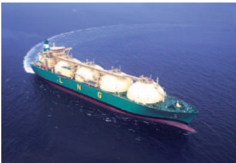
Figure 1: Spherical tank LNG carrier [1] with a capacity of 137 000 m 3 .
