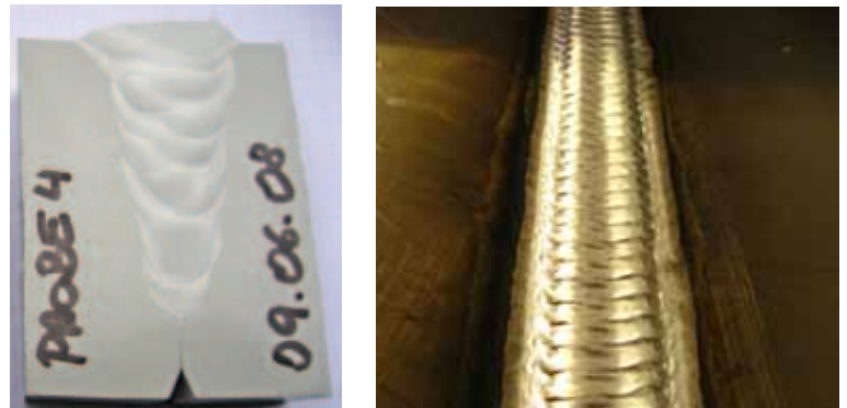
Figure 14: Initial results at reducing the number of weld layers – cap layer appearance (left) and transversal macro section (right) [7].
