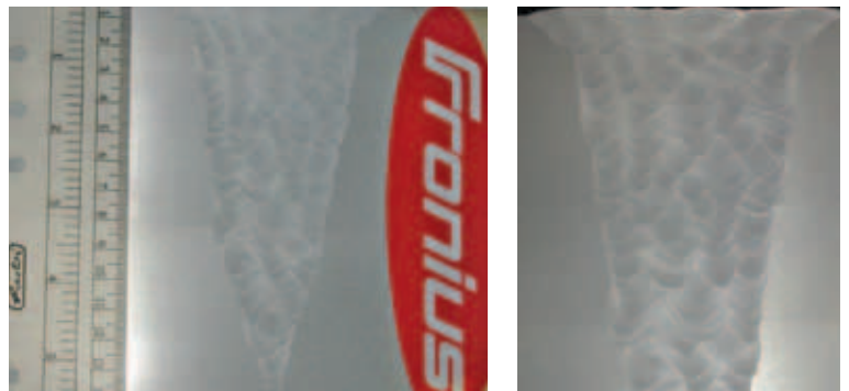
Figure 7: Heavy section aluminium plate ( t = 150 mm) manually welded using single wire narrow gap GMAW-P [7].
