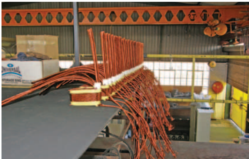
Inverter welding transformers are much smaller and cheaper than the traditional 50 Hz welding transformers. These being manufactured at Reeflex have only three turns on each side and each can cope with 5,0 kW of output welding power.
