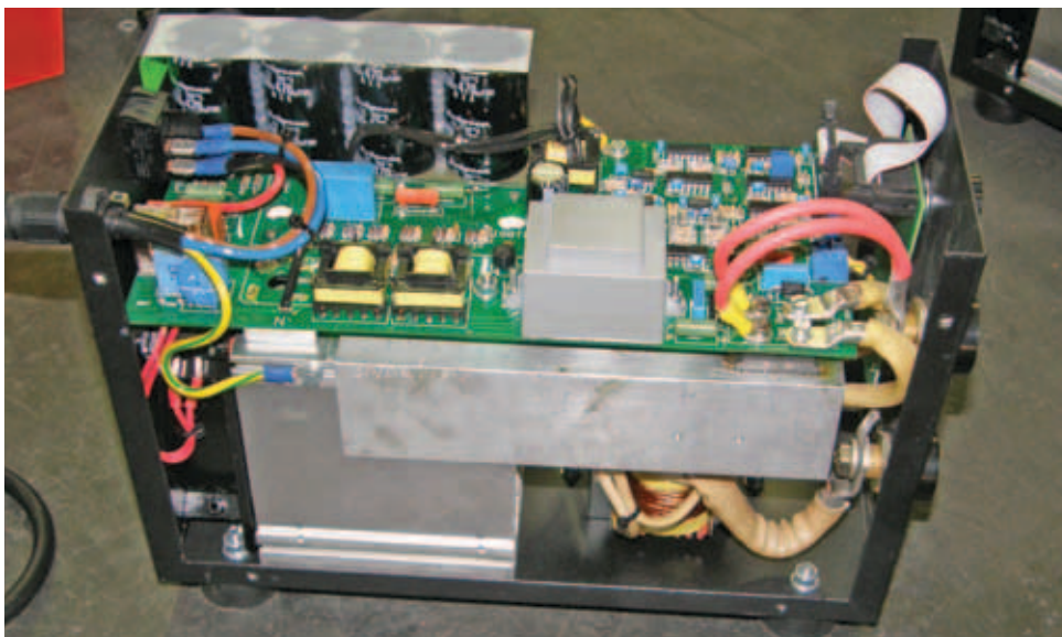
The smallest (6,0 kg) Reeflex machine, the 140, 150 or 160 A units for single phase operation.
