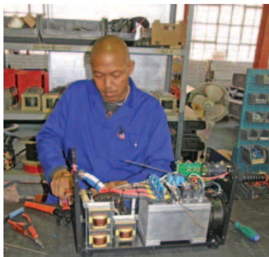
A 400 A stick/TIG inverter welding machine being assembled by Vincent Barns at Reeflex Welding in Strydompark.
