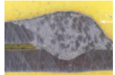
A weld seam and a micrograph of lap joint in 0,8 mm CrNi-steel robot welded at 100 cm/min using the microMIG process. Wire: ER 307 Si 1,0 mm. Gas: 98% Ar 2% CO 2 .
