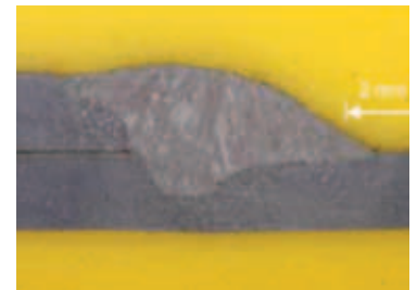
A weld seam and a micrograph of lap joint in 2,0 mm CrNi-steel robot welded at 100 cm/min using the microMIG process. Wire: ER 430 CB 1,0 mm. Gas: 98% Ar 2% CO 2 .
