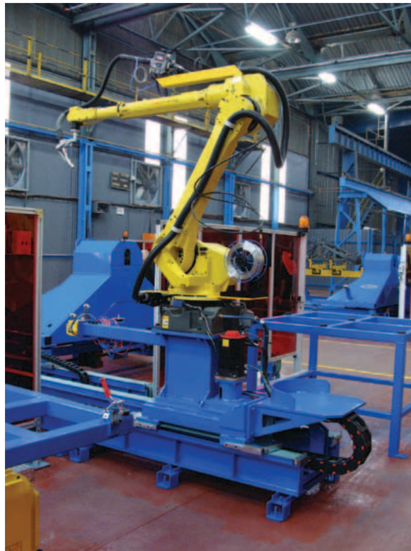
The six-axis welding robot travels on a linear rail to access each of the four workstations.
