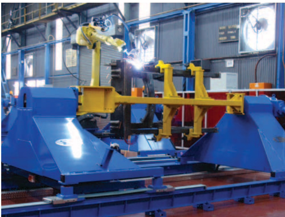
A wheel module component being welded at the front-end workstation.
