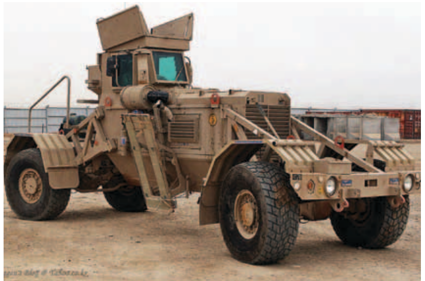
The South African-designed and manufactured mine detection vehicle that can detect mines while travelling at 25 km/h. (Image from: img.blog.yahoo.co.kr/ybi/1/24/56/shinecommerc ).
