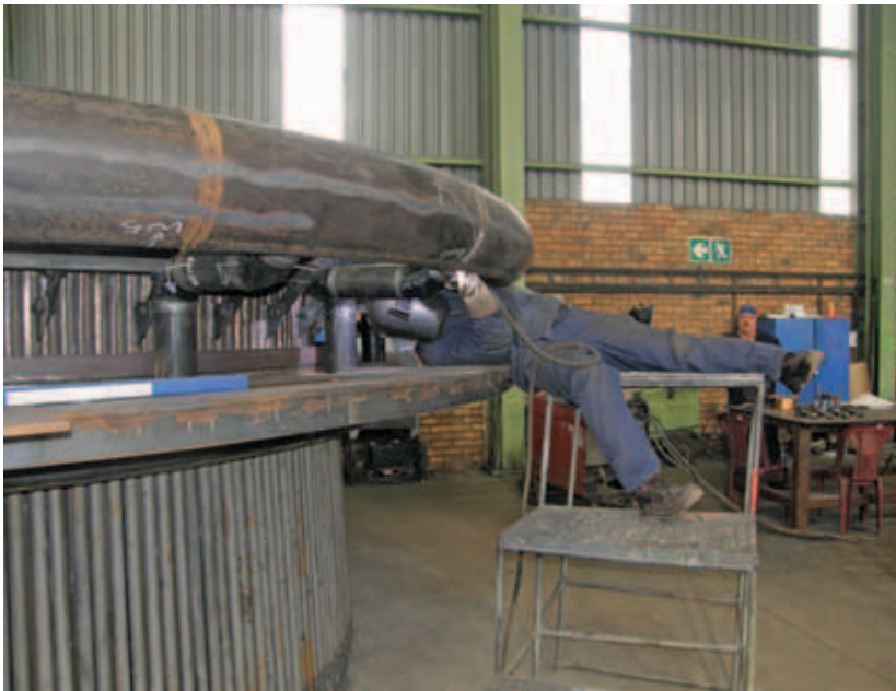
A highly-skilled TIG welder working on an energy recovery hood at ISO 3834 certified welding fabricator, Engski Manufacturing.
