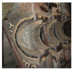
Stoody manufactures products such as the Stoody 1102 solid core electrode, which has an all weld metal composition and physical properties similar to those of H-12 tool steel. This makes it ideal for repair welding of components such as bearing
