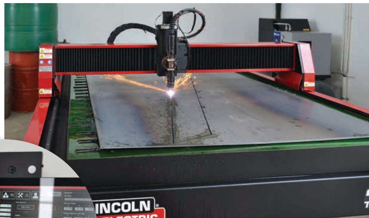
Above: With a bed size of 1.25x2.50 m, Tsipe Engineering's Torchmate 4800 cuts standard sheet of 1.2x2.4 m and the FlexCut 125 can cope with thicknesses of up to 25 mm.
