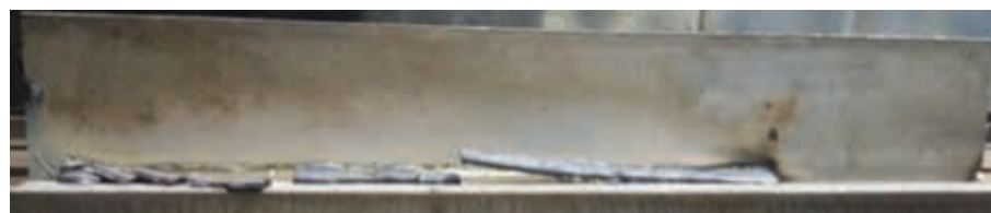
Photo1: Nice welding appearance and easy slag detachability for Clearinox.
