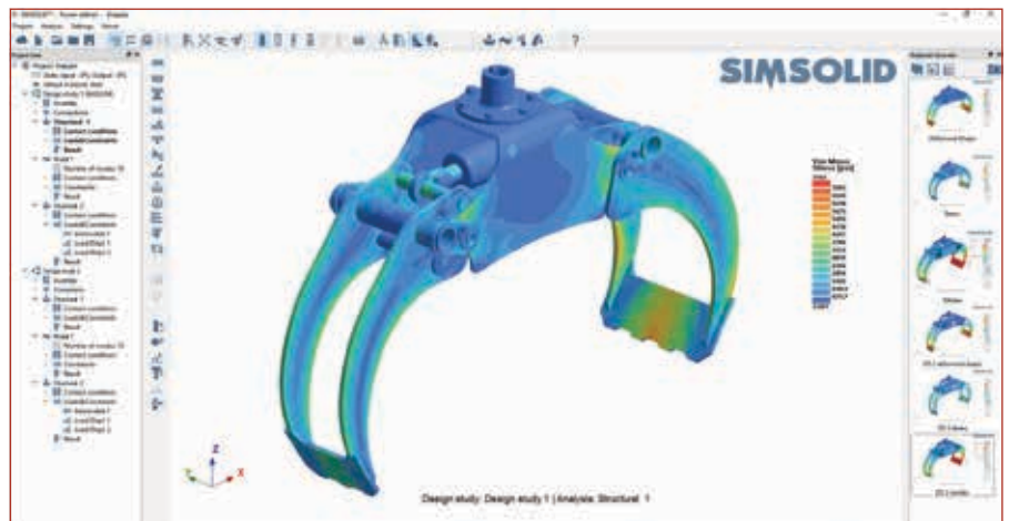
A SimSolid analysis result for a grapple hook.
