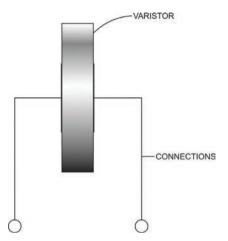
MOV arrestors are used in Type II and Type III arrestors and since this varistor is connected directly to the terminals, a small current flows continuously between them. As the voltage increases, the current also increases slightly until, at breakdown, a sudden and high current flows through the disc and persists until the voltage drops to a value below the breakdown level.
