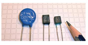
The thermal disconnector is a crucial component in the surge protection circuit as it prevents a fire developing within the MOV assembly after it has absorbed repetitive surges over its lifetime.
