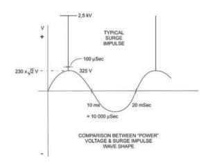
A typical voltage surge or spike has a peak of 2.5 kV with a 1.2 micro-second (1.2/1 000 000 of a second) rise time and a fall to 50 % of the peak value in 50 microseconds.
