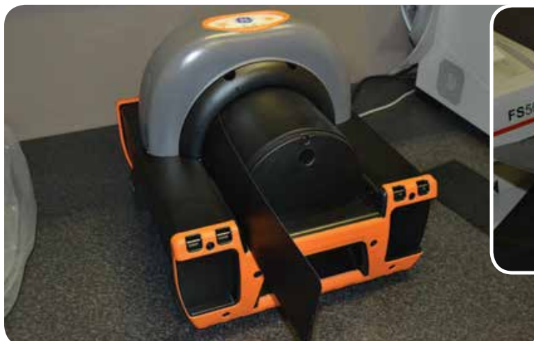
Left: The Institute's CR scanner used to transform the latent image captured in the imaging plate into a digital radiographic image. Above: A phosphor-coated digital imaging plate used for CR digital radiography.
