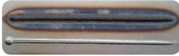
For full penetration welds, the underside of the weld needs to be purged to keep oxygen and hydrogen away from the HAZ and the molten metal.
