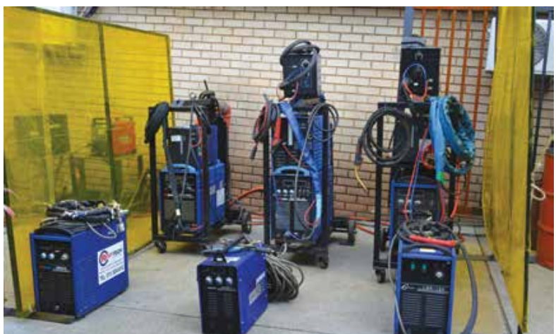
UniPower customises machines for South African rental customers by enlarging the heatsinks, increasing the airflow and isolating the PC boards from the dust-bearing airflow.
