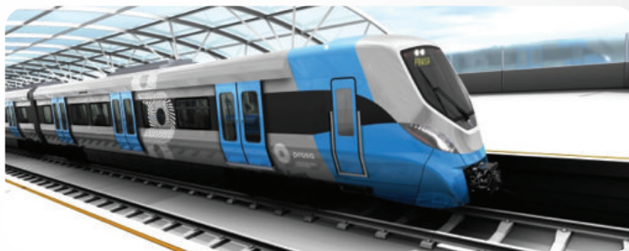
PRASA will be supplied with the X'Trapolis Mega. A new X'Trapolis train was developed by Alstom to fit South Africa's 1,067m gauge.
