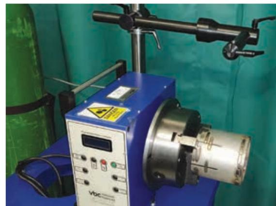
The welding was carried out on pieces of 22-inch OD, 0.5-inch wall thickness, 316 stainless steel tubing manipulated using a VBC Model W Assisted Hinge turntable.
