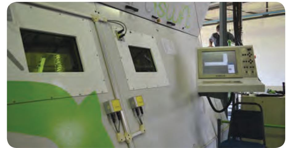
A purpose-developed controller gives the flexibility to control and optimise every individual parameter – even the functional material densities and strengths in different places of a component.
