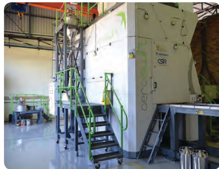
The Aeroswift powder bed fusion LAM machine was designed for big powder volumes of up to 2 000×600×600 mm, predominantly for manufacturing aerospace components in titanium.
