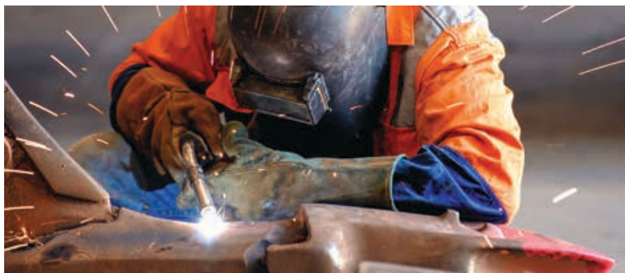
Oerlikon consumables have been optimised to reduce impurities and diffusible hydrogen in order to more efficiently overcome the cold cracking hazard.
