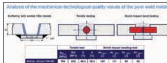
Figure 10: Normative specification for determining the mechanical properties of the weld metal.
