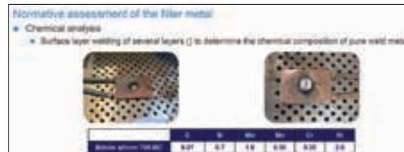
Figure 9: Normative requirement for determining the chemical composition of welding consumables.
