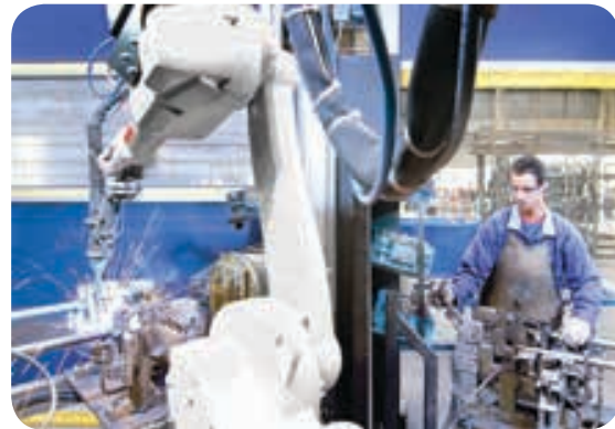
Welding is a key growth area for robot use, particularly among Tier 1 and 2 automotive components manufacturers.
