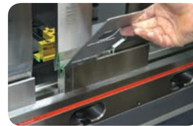
Bystronic press brakes sense the pressure required by each component and adjust to ensure that the angle required is achieved.
