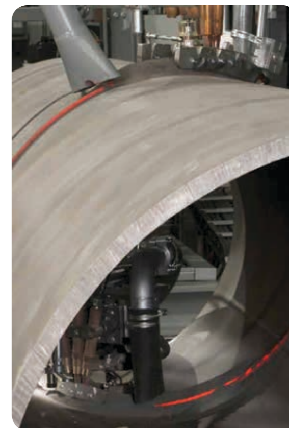
The advantages of SAW over other welding processes include: high deposition rates; typically deep penetration; high operating factors, due to the mechanised nature of the process; and low hydrogen levels in deposited weld metal.
