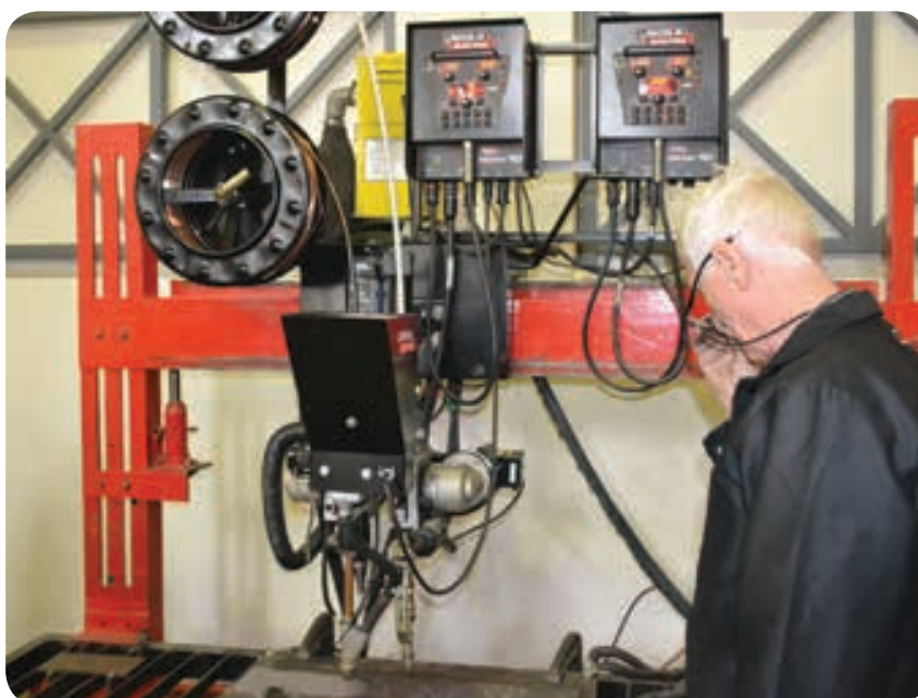
Josef Henning demonstrates submerged-arc welding using a Power Wave 1000 SD in dc constant current mode.
