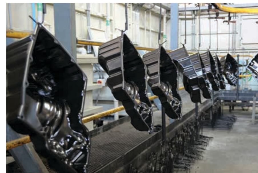
From a quality perspective, the process offers 100% coverage of complex parts with a uniform film thickness, giving benchmark corrosion protection to metal components.
