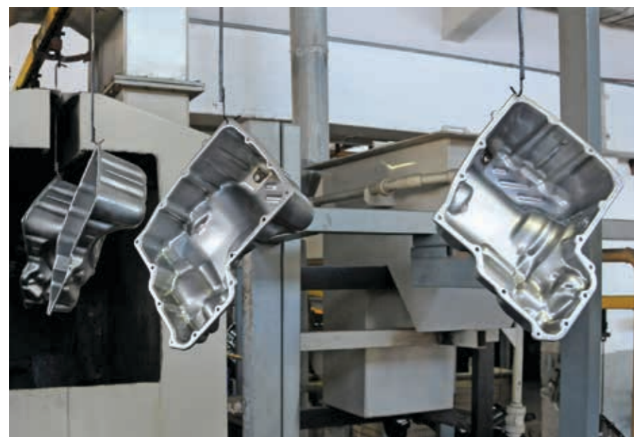
In the first stages of the fully automated electrocoating process, the parts are cleaned and phosphated to prepare the metal for the paint application.
