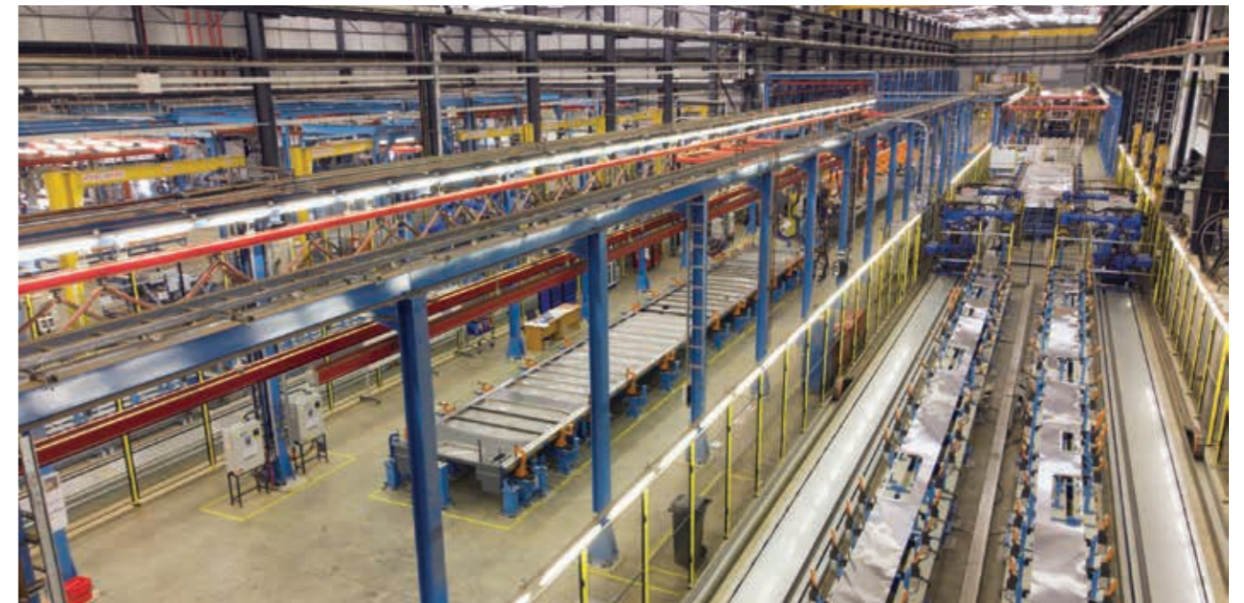
A view of Gibela's car body shell main sub-assembly area showing the sidewall (far left), under-frame (centre); and roof/letter-board (right) welding assembly areas.
