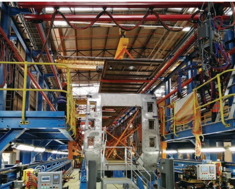
The Cathedral or main framing line at the flagship Gibela Dunnottar train-manufacturing plant, where the under-body, end-frames, roof and sidewalls are loaded together and framed to complete the shell.
