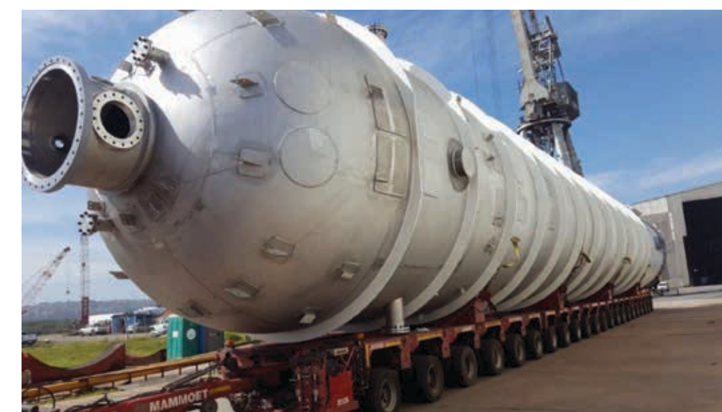
NDE's winning entry in the Duplex Stainless Steel category, the Mondi Oxygen Reactor, which, according to the judges, "demonstrates consistent mastery of the use of duplex materials".
