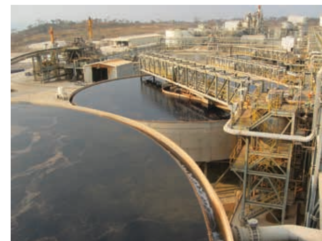
35 metre diameter CCD thickeners in a copper leaching circuit.
