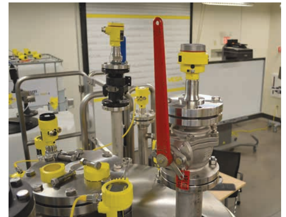
After reports of success on valves in the field, VEGA tested the VEGAPULS 64 in its Learning Centre Lab and saw impressive results. The tests revealed that level measurement through a valve is easy with 80 GHz devices and impossible with GWR.
