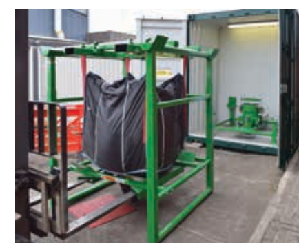
Above: The bulk bag and lifting frame of the BFF-C-X Bulk-Out™ split-frame bulk bag discharger are forklifted onto the stationary discharger frame inside the container.
