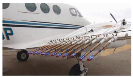
WAS is equipped with a Piper Chevenne twin turbine aircraft fitted with a flare deployment system for cloud seeding.
