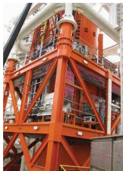
The from-the-deck view of the Seabed Tool (SBT), a world-first advanced sub-sea sampling system aboard the mv SS Nujoma.
