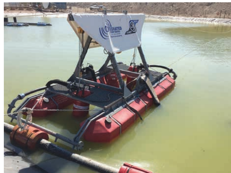
Designed to clean lined process ponds, the Slurry Sucker system does not require submersible pumps with cutter heads to agitate the settled sludge and, due to the design and engineering of the dredge head, it is able to operate while the pond is online.
