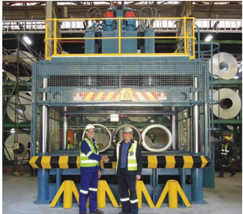
The pup-coil press built for Hulamini Aluminium uses a control strategy for a four-cylinder hydraulic press that always ensures the press remains parallel.
