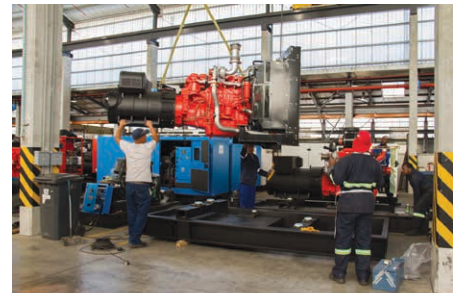
Packaging and assembly of custom-engineered generator set solutions underway at the Zest WEG manufacturing facility in Cape Town.
