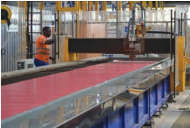
Left: To improve the accuracy, consistency and safety of liner cutting, Weir Minerals uses a CNC AquaCut water jet cutting system to cut Linatex sheet into the rubber shapes required. Right: Linatex premium rubber sheeting is passed through a buffing machine to roughen the surfaces.
