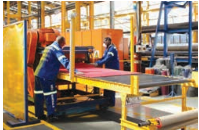
Left: To improve the accuracy, consistency and safety of liner cutting, Weir Minerals uses a CNC AquaCut water jet cutting system to cut Linatex sheet into the rubber shapes required. Right: Linatex premium rubber sheeting is passed through a buffing machine to roughen the surfaces.
