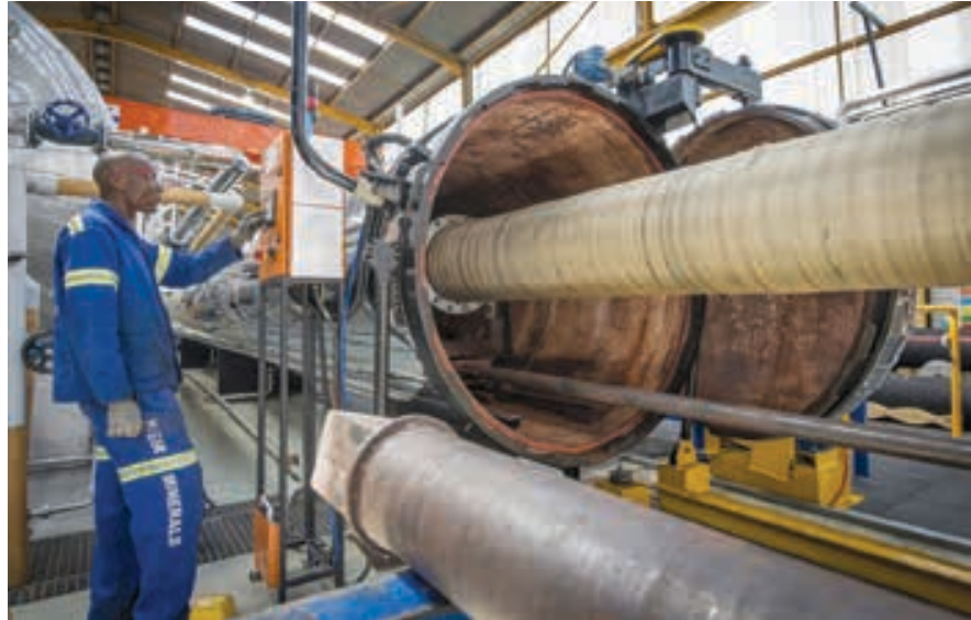
One of three autoclaves at Weir Minerals Africa's Alrode plant used to cure rubber hoses as part of the manufacturing process.
