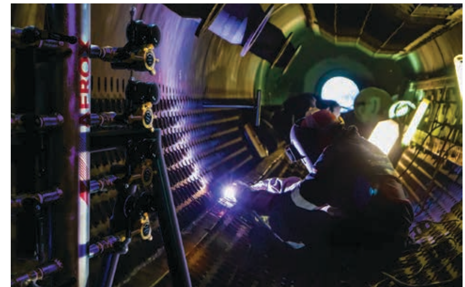
Each welder simply connects his or her gas hose to a point on the MUPP for regulated access to the shielding gas needed.
