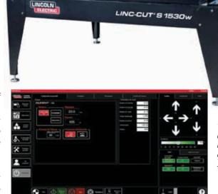
The VMD user interface allows you to control the machine and is installed on an easy-to-use 16/9multi-touch screen
