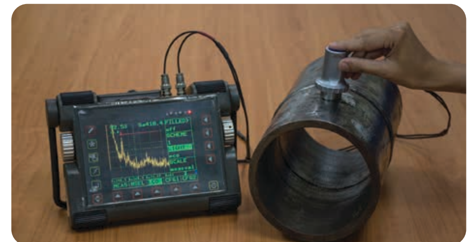
A weld on a steel pipe being inspected using the non-destructive ultrasonic testing technique.
