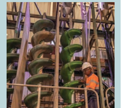
Hlayisi Baloyi, applications engineer at Multotec, has been conducting extensive test work on Multotec's new SC25 spiral concentrator using ferrochrome samples from numerous mines.
