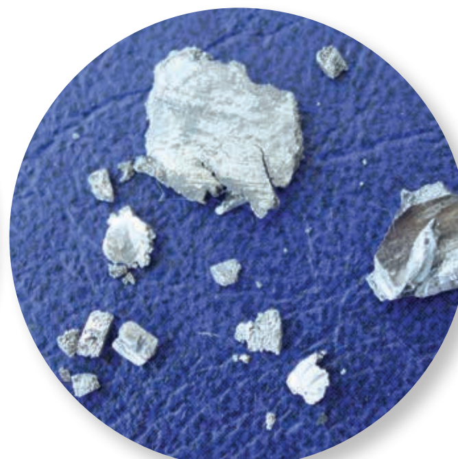
Wear debris from a magnetic plug, in the right hands, speaks volumes about the state of the equipment, without having to take it off-line for disassembly.
