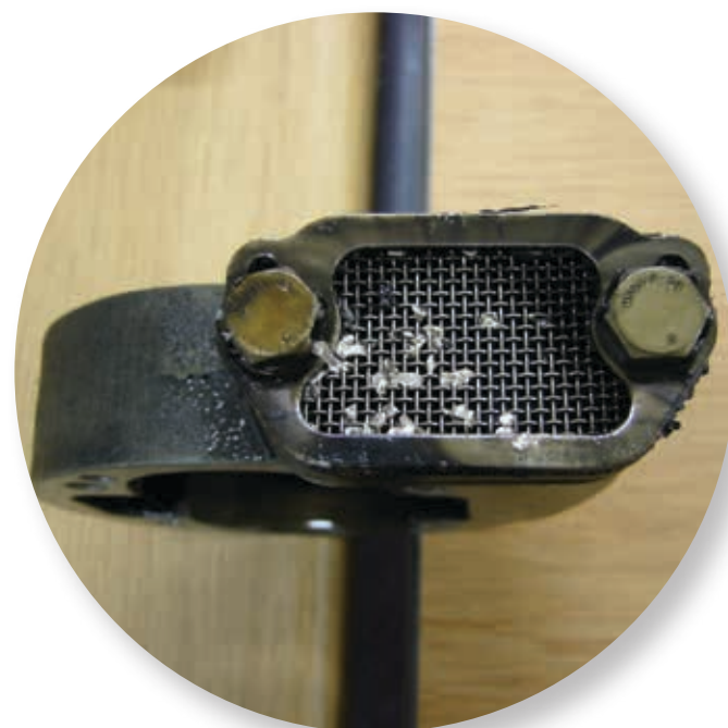
Dismantling a used oil pump strainer filter to recover wear debris for analysis, although messy, is not as messy as having a machine breakdown
