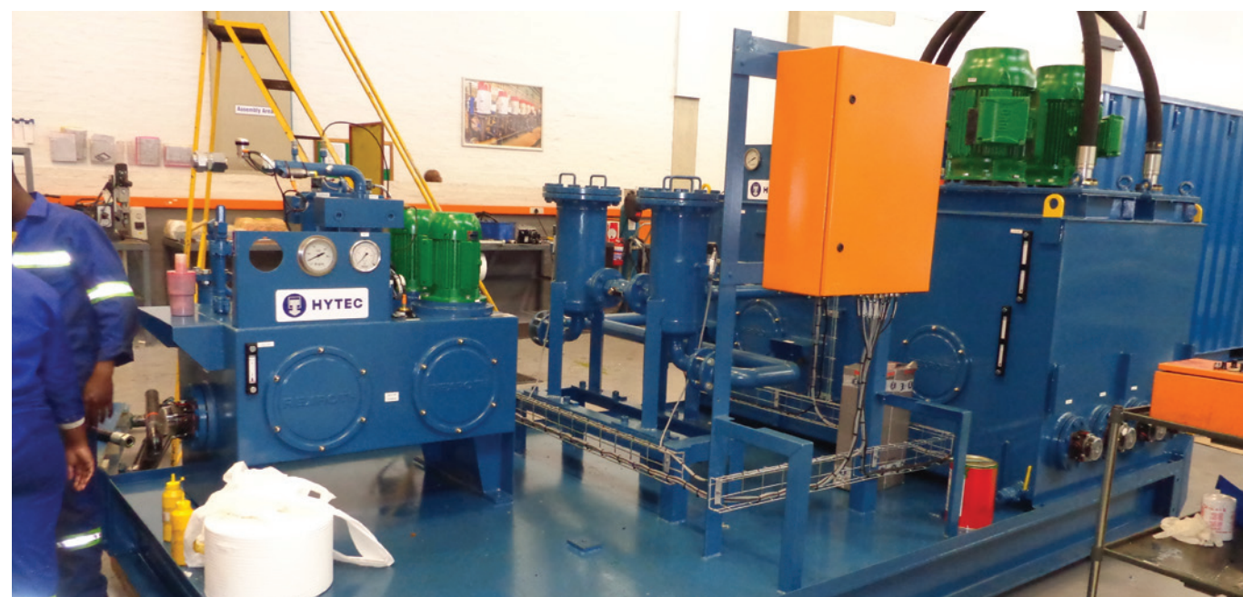
Bosch Rexroth pump and motor test stations, from 90 kW to 600 kW, are connected to CADASYs, Bosch Rexroth's data acquisition and recording system.
