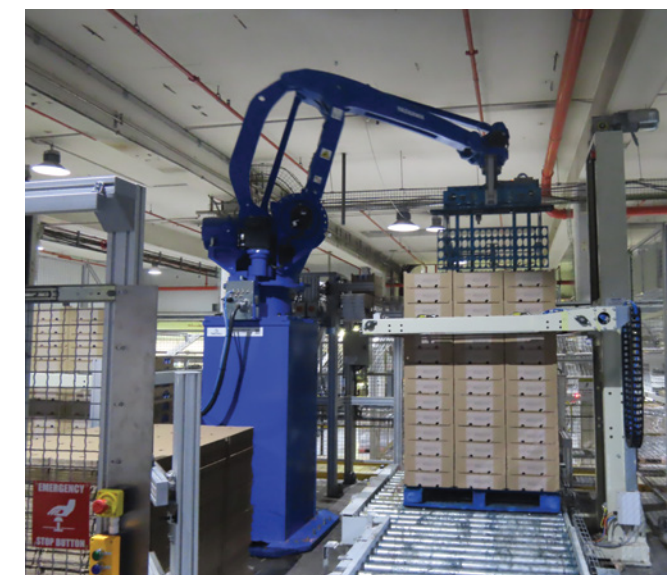
Left: Tectra Automation's solution increased pallet consistency across Danone's product range. Right: Tectra Automation's solution for Danone included Yaskawa palletising robots, state-of-the-art shrink-wrapping machines, conveyor systems, light curtains, safety sensors and scanners.
